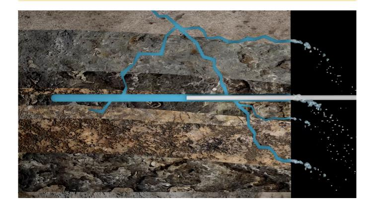
Water ingress into an underground mine can represent a major risk if not recognised and rectified. It can compromise the integrity of the ground support system while an uncontrolled inrush of water can hinder any further progress in the operation.
