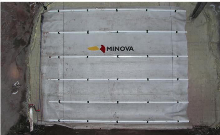
**Minova's QBC blind is an easy to install ventilation device that allows for stopping of airflow to or from the area of a mine that may require access at a later stage.**
